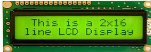
**Gambar 2.8** Display LCD 2x16
