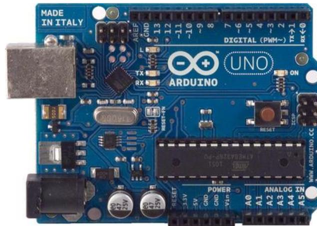
Gambar 2.1. *Board* Arduino Uno
