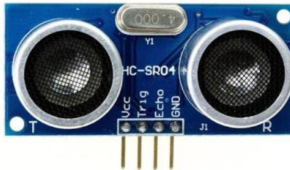
Gambar 2.6 Sensor Ultrasonik HC-SR04
