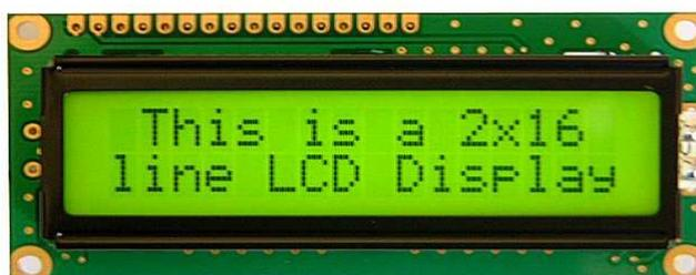
**Gambar 2.20** *LCD* 16x2
