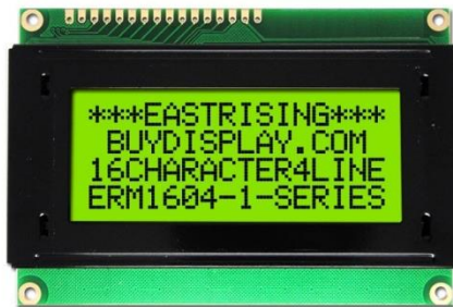
Gambar 2.17 LCD ( Liquid Cristal Display )
