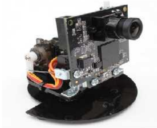
Gambar 2.7. Pixy CMUCam5 ( http://cmucam.org/projects/cmucam5 , 2017)
