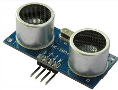
**Gambar 2.22** Sensor Ultrasonik HC-SR04
