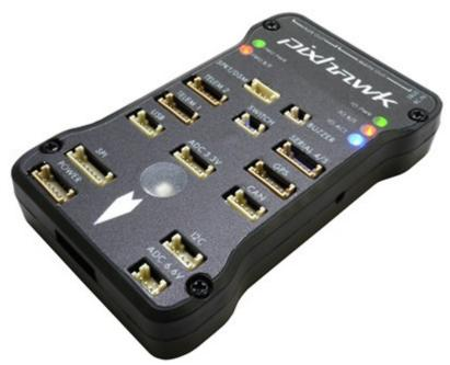
Pixhawk is an advanced autopilot system designed by the PX4 open-hardware project and manufactured by 3D Robotics. It features advanced processor and sensor technology from ST Microelectronics® and a NuttX real-time operating system, delivering incredible performance, flexibility, and reliability for controlling any autonomous vehicle.
