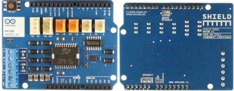
Arduino Motor Shield R3 Front
