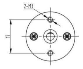
Fig. 2. Front view of the JGA25-370RC DC gearmotor
