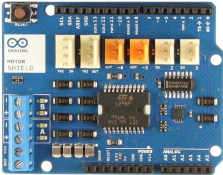
Arduino Motor Shield R3 Front
