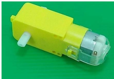
Gambar 2.11 *Motor DC + Gear Box*
