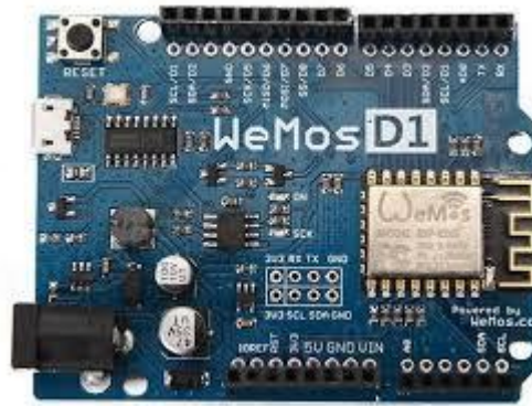
Gambar 2.2 Modul Wifi Wemos ESP8266
