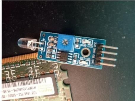
Gambar 2.3 Sensor Photodioda
