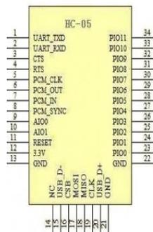
**Gambar 2.12** Pin out Modul *Bluetooth* HC-05
