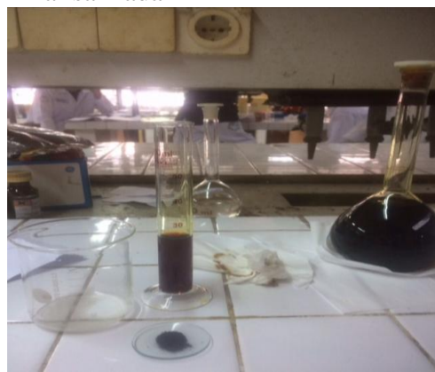
Gambar 33. Penentuan daya serap iod
