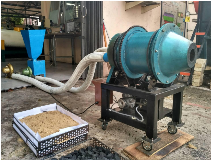
Pulverizer Coal Burner
