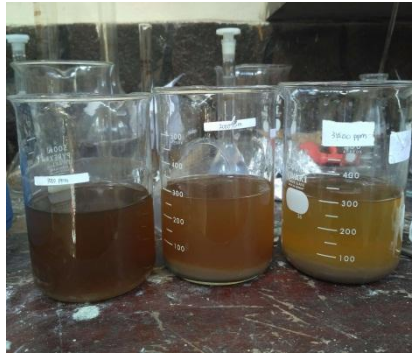
Gambar 13. Penentuan Koagulan Optimum 1000 ppm, 2000 ppm, & 3000 ppm
