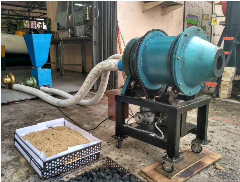
Pulverizer Coal Burner
