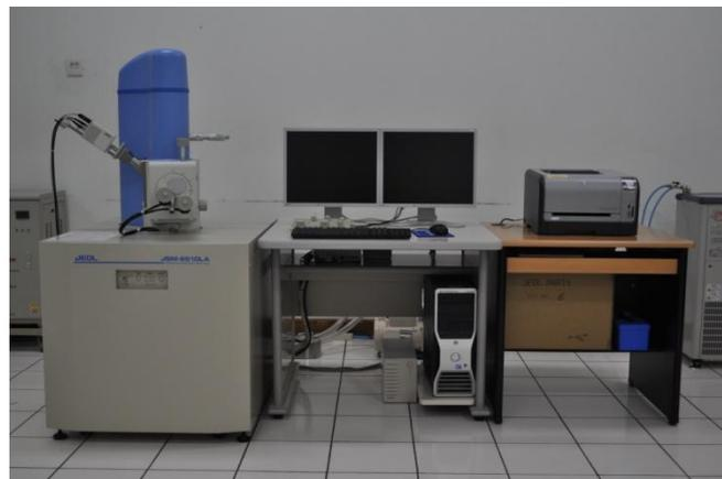
Gambar 2.4. Alat SEM Tipe *JSM-6510A/ JSM-6510LA (Analytical / Analytical low vacuum SEM)*
