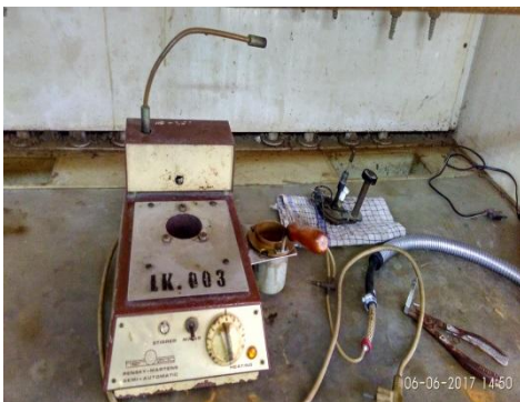
Gambar 21. Flash Point Tester
