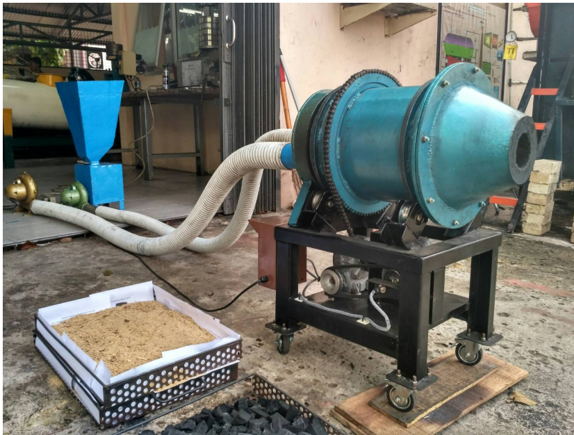
Pulverizer Coal Burner
