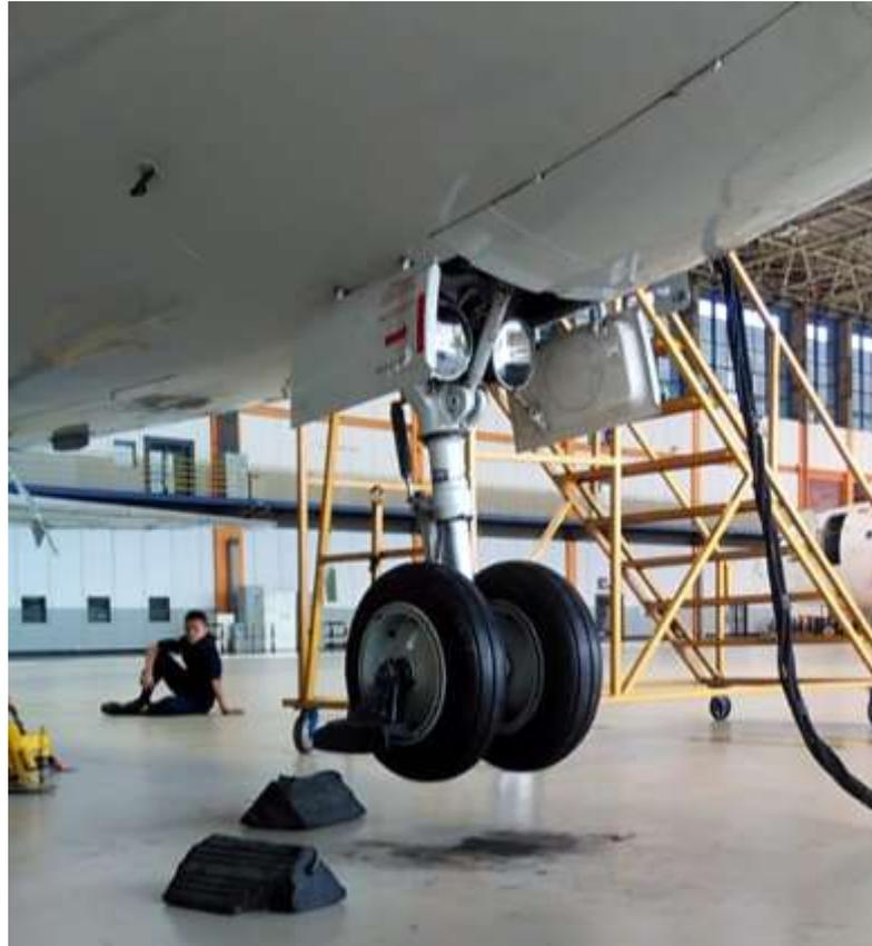
**Gambar 2.1** *Landing gear extension*
