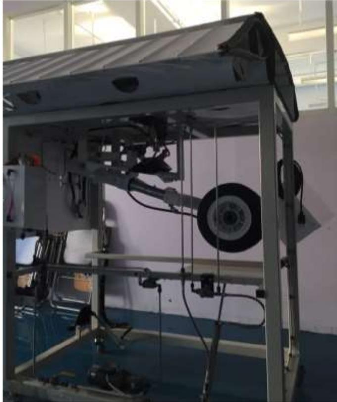
**Gambar 2.3** Simulator *landing gear extension* dan *retraction*
