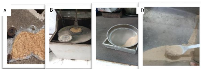
Fig. 1. Preparation of ultimate and proximate testing of rice husks (A) Rice husks material, (B) Pulverizer (C) Sifting (D) Rice husks size reduction
