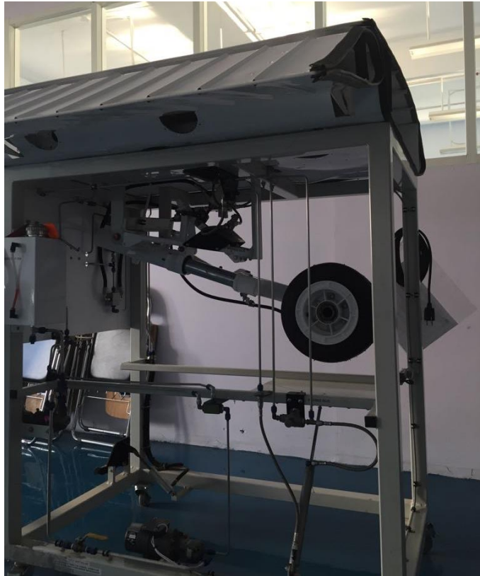
Gambar 2.3 Simulator landing gear extension dan retraction Sumber: Simulator landing gear Polinema
