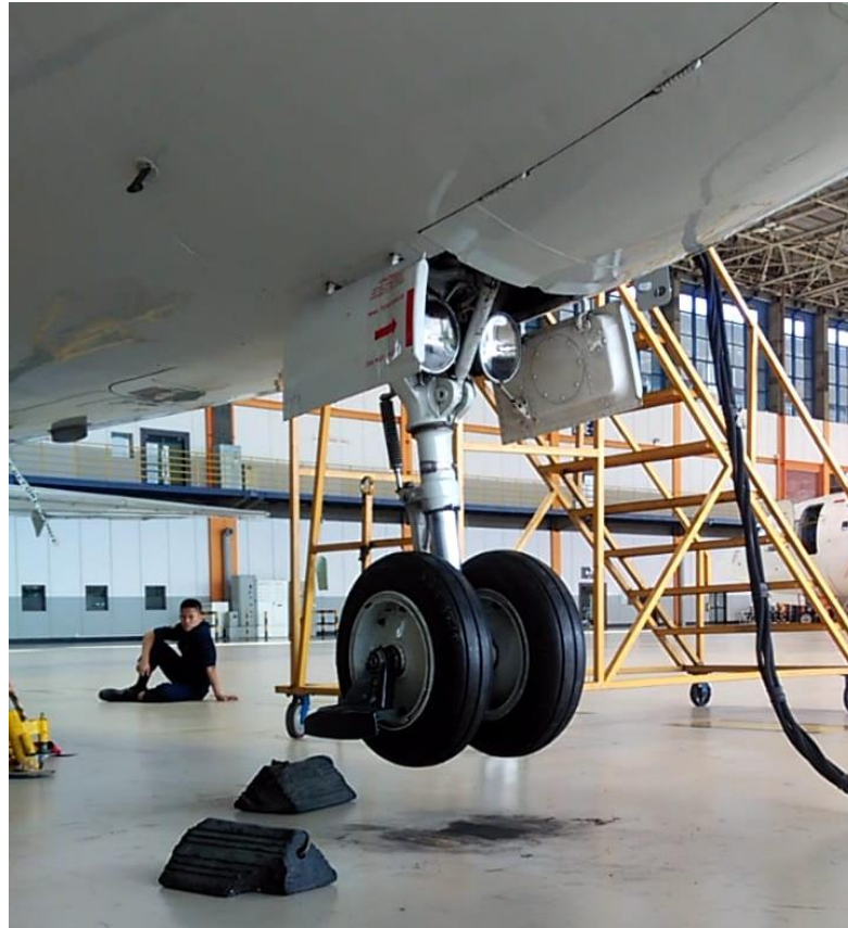
Gambar 2.1 Landing gear extension Sumber: Pesawat DC-9 Hangar 2 GMF Aeroasia
