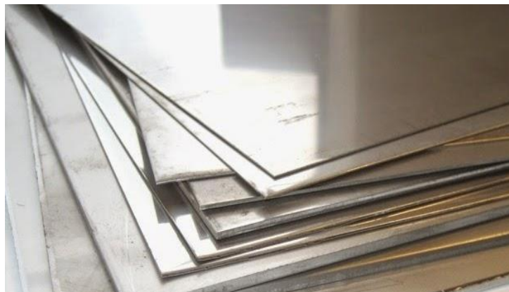
Gambar 2.6 Plat Stainless Steel (Sumber: Lit. 18)
