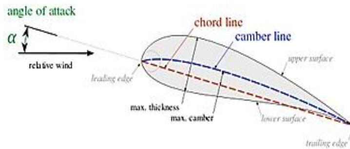
Gambar 2.22 Bagian-Bagian *Airfoil*
