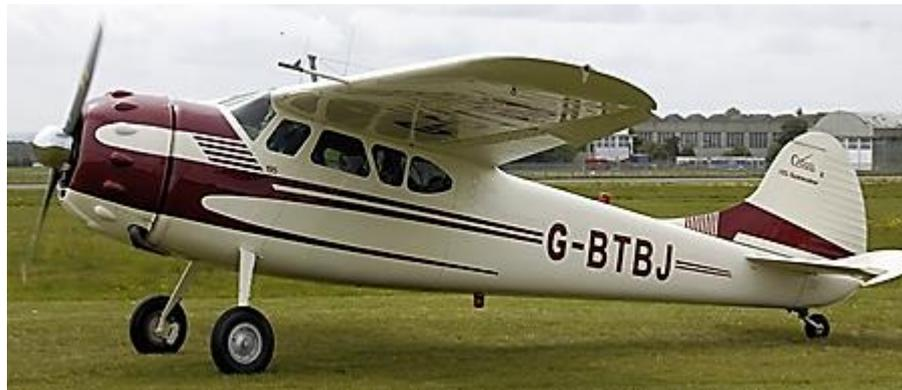
Gambar 2.15 *Landing Gear Conventional*
