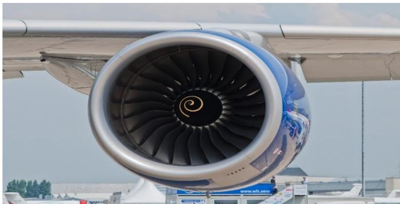
Gambar 2.11 *Engine Airbus A-320*
