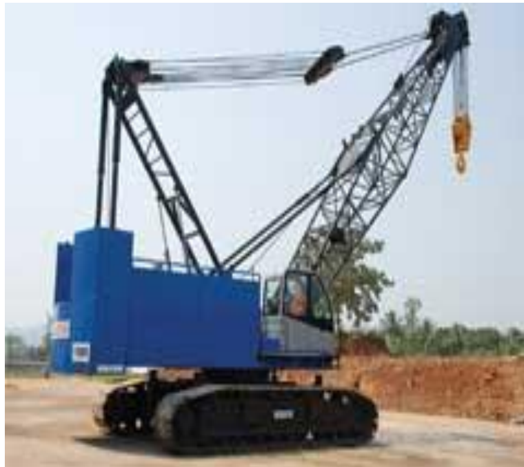
Gambar 2.3 Crawler Crane in Hold Position
