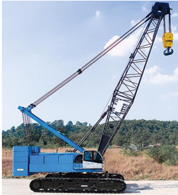
Gambar 2.4 Crawler Crane in Raise Position
