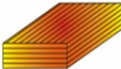
Gambar 2.1 *Continuous fiber composite*
