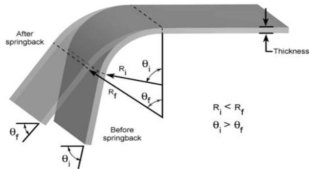
Gambar 2.8 Proses *Bending*
