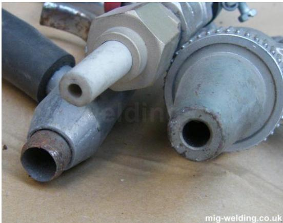
Gambar 2.10 *Nozzle sandblasting*
