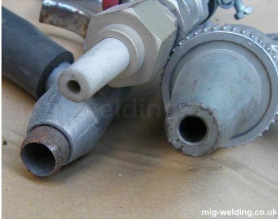
Gambar 2.9 Nozzle *sandblasting*
