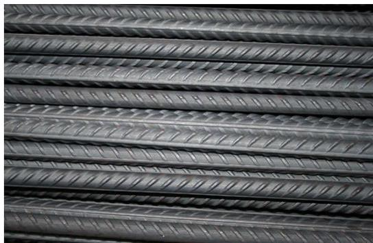
**Gambar 2.5 Baja Tulangan Beton Sirip**
