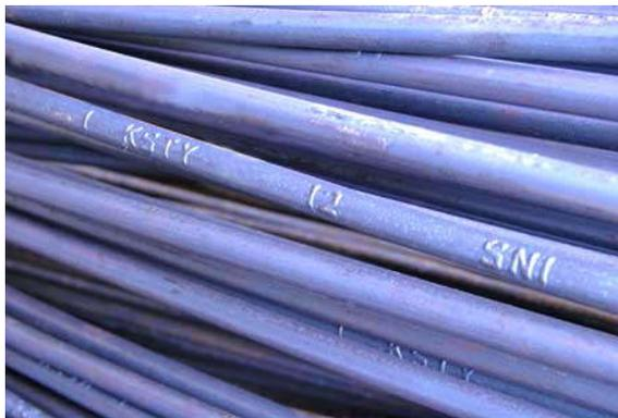
**Gambar 2.4 Baja Tulangan Beton Polos (BjTP)**
