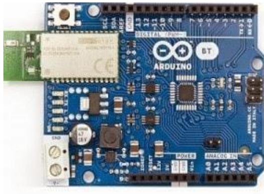
**Gambar 2.16 Arduino BT**
