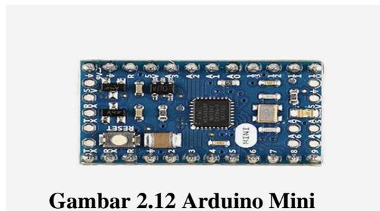
**Gambar 2.12 Arduino Mini**
