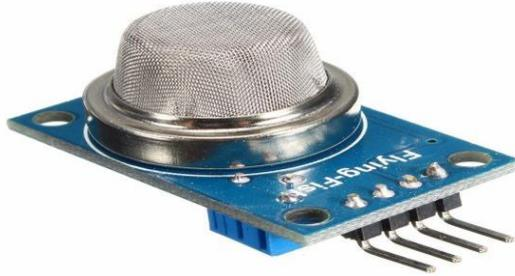
**Gambar 2.2 Sensor Gas MQ-9**
