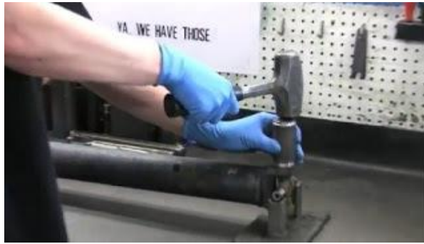
Gambar 2.24 Melepas Bearing Cup
