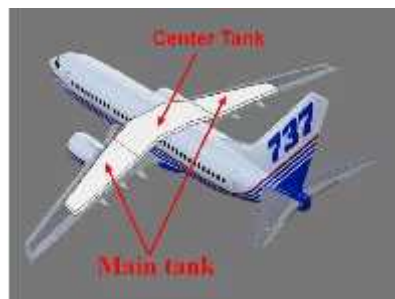
Gambar 2.5 Boeing 737-800NG Fuel Tank (Sumber : https://veeone120184.files.wordpress.com )
