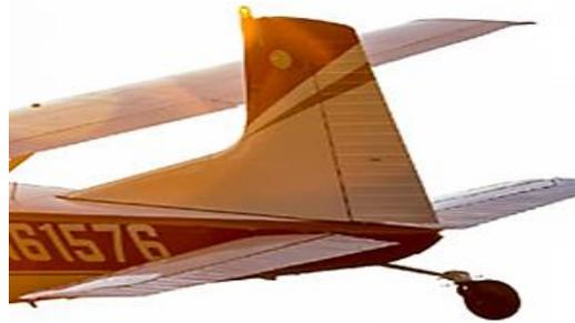
**Gambar 2.8** *Empennage* Pesawat Cessna 180 Skywagon
