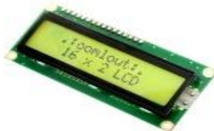
**Gambar 2.28** LCD (*Liquid Crystal Display*)
