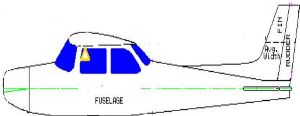
**Gambar 2.13** *Flight Control Surface* Tampak Samping
