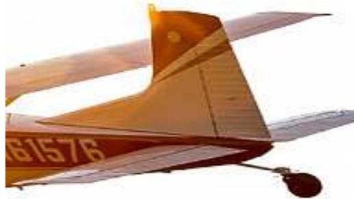
**Gambar 2.8** *Empennage* Pesawat Cessna 180 Skywagon
