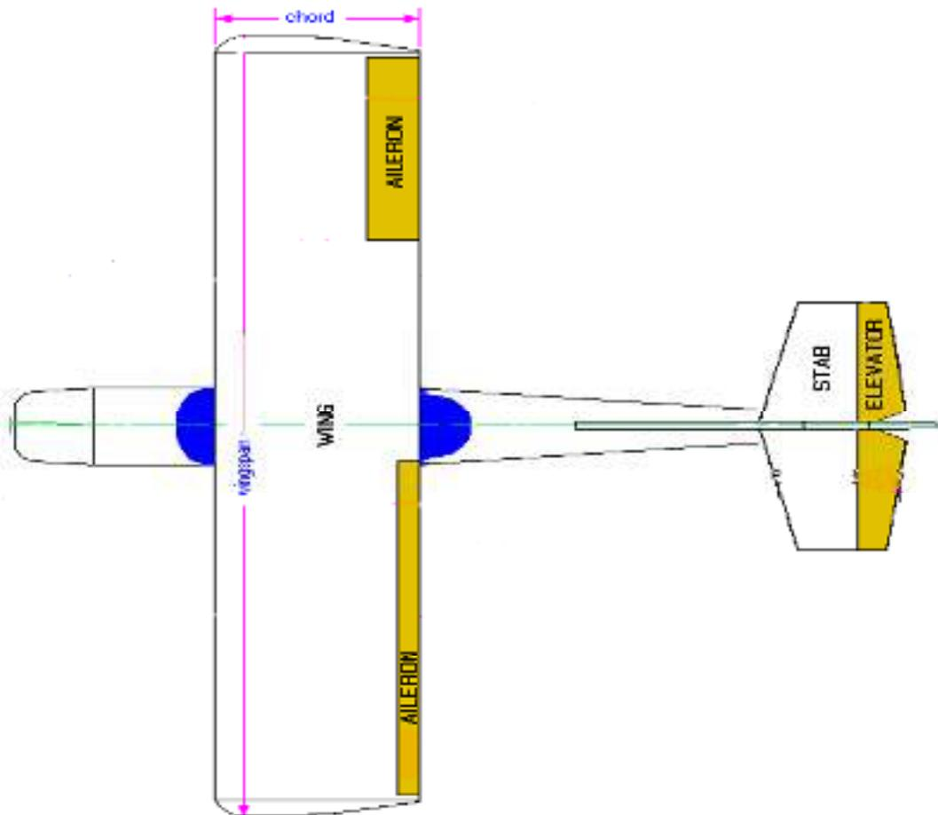
**Gambar 2.12** *Flight Control Surface* Tampak Atas
