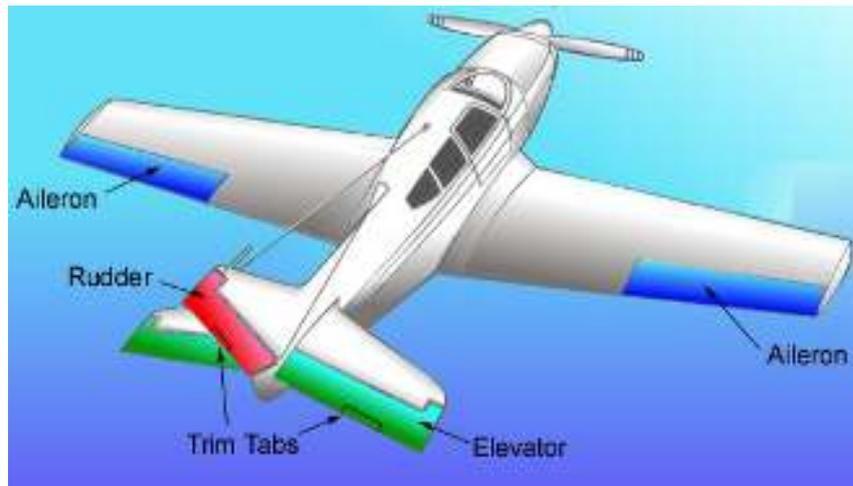
**Gambar 2.14** *Flight Control Surfaces*
