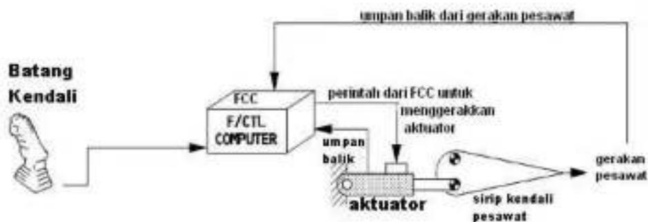
**Gambar 2.24** *Fly By Wire Basic Layout*
