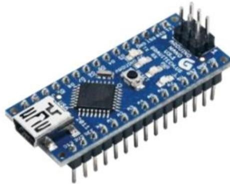
Gambar 2.2 Arduino Nano328p
