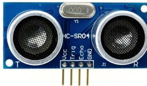
Gambar 2.6 Sensor Ultrasonik HC-SR04
