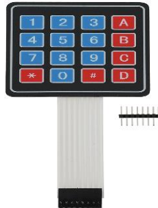
Gambar 2.10 Keypad matrik 4x4
