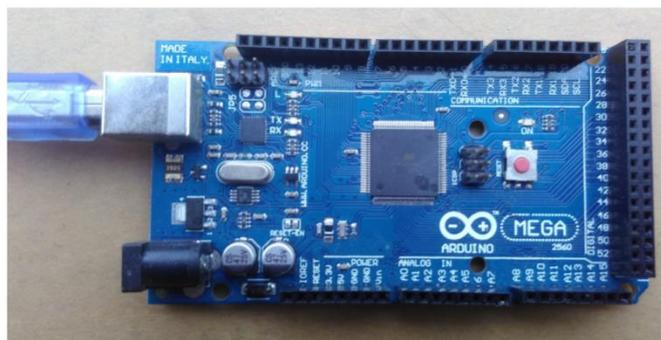
**Gambar 2.6 Arduino Mega2560**
