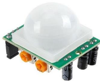
**Gambar 2.10** Tampilan Depan Modul HC-SR501 PIR Motion Sensor
