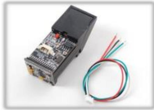
**Gambar 2.2 *Fingerprint Sensor***
