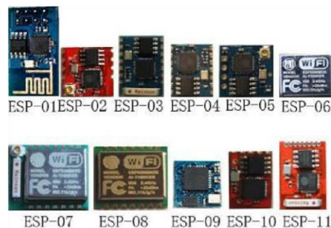
Gambar 2.7 Macam macam jenis modul ESP8266
