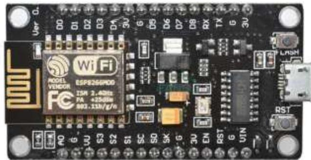
**Gambar 2.2** NodeMCU ESP8266
