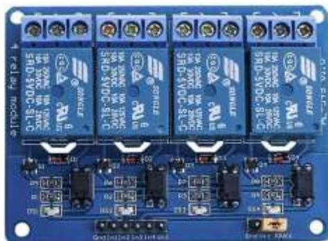
**Gambar 2.3** Module Relay 4 Channel
