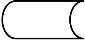
A horizontal oval shape with a semi-circular end on the left and a semi-circular indentation on the right, representing a disk.         | Simbol disk storage, menyatakan input berasal dari disk atau output disimpan ke disk. |
