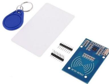
**Gambar 2.1** RFID-RC522 Dan RFID Tag
