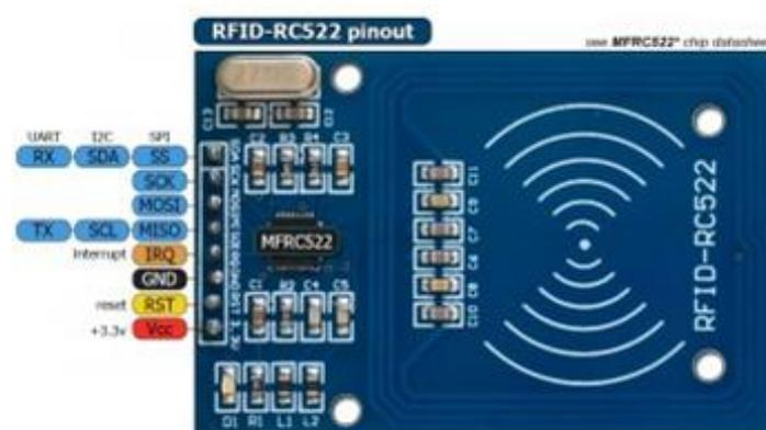
**Gambar 2.5** Modul RFID Reader RC522
