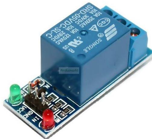
**Gambar 2.12** Modul *Relay 1 Channel*
