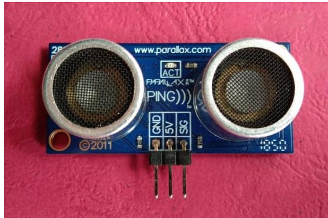
**Gambar 2.1** Sensor PING Ultrasonik
