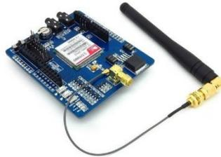
**Gambar 2.4 Tampilan Modul GSM SIM900A**
